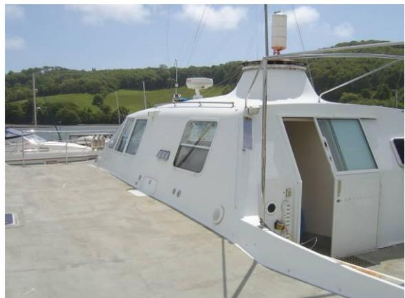
I therefore assume the turret is strong enough to mount an unstayed mast directly on the turret. A hinged base plate can then be used to allow the mast to be lowered without the use of a crane. The mast length needs to be less than the 17.4 meter length of Planesail in order to avoid any overhang fwd or aft when lowered.
